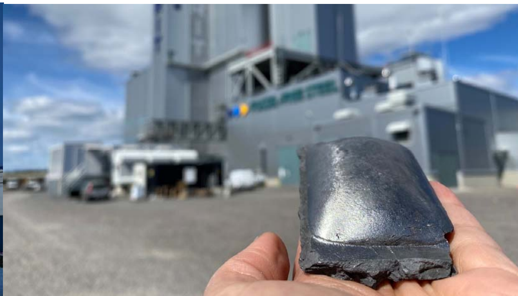
A piece of fossil-free sponge iron with the Hybrit pilot plant in the background. Credit: Hybrit
